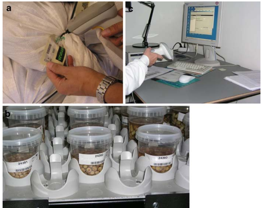
Fig. 4 The use of bar coding for sample registration (a), sample processing (b), and entering the final test results (c) ensures a high degree of sample integrity and quality of the test result
